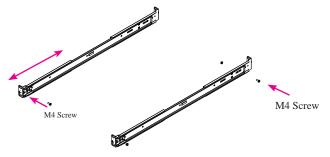
3 Mounting the rear ear bracket to rear side of rail. Adjust the rear ear bracket according to depth of your cabinet. If a screw hole is available, secure ear bracket to outer rail with a M4 screw. If only open slot is available, secure rear ear bracket with outer rail with M4 screw and M4 nuts. Do not tighten screw yet.
