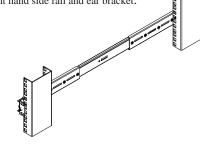
Attaching center rail to right side of your equipment. Make sure at lease 2 screw holes are aligned. Secure center rail to shelf with M4 screws to complete your installation.
